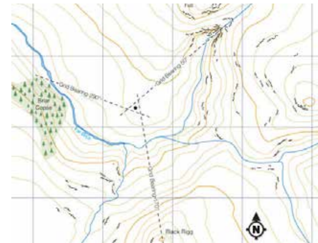
PUTTING IT INTO PRACTICE See known features locating the taker within a triangle. © MTUK/VG 2012
