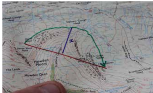
The distance x (blue line) is roughly the extra distance run by contouring compared to the direct route (red) © MTUK/VG 2012
